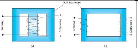
Working: When an alternating voltage is applied to the primary, the resulting current produces an alternating magnetic flux which links with the secondary and induces an e.m.f. in it.
